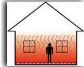
Heat Profile with Radiant Floor Heating
